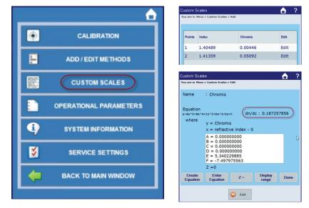
This method gives the identical result as the more laborious plotting of multiple points, and both agree with the value published by the GPC vendor, namely 0.187 and 0.188 vs 0.185.
